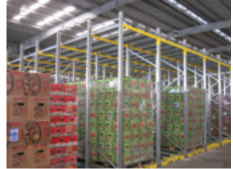
Pallet flow racking systems are a FIFO (First In First Out) dynamic storage system. Gravity flow racking maximizes storage space by minimizing aisles.
