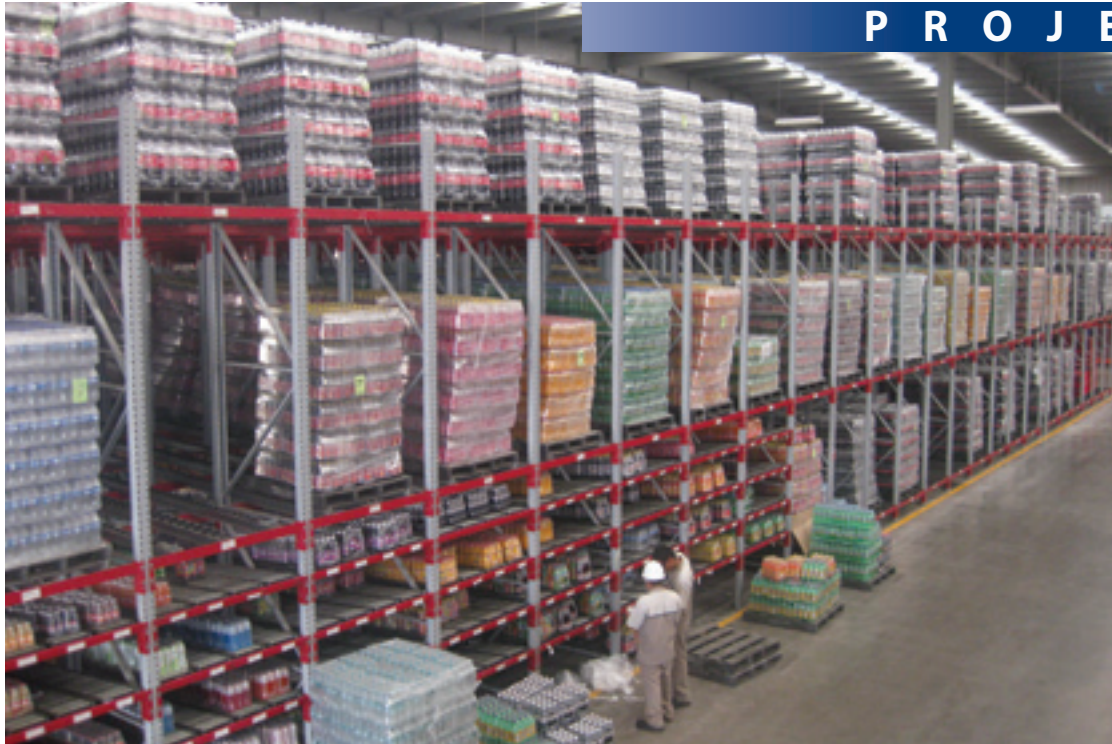
Two sections of gravity flow 14 pallets deep 1,500 pallets stored at dynamic racks levels. Flexible to operate with plastic and wood pallets.
