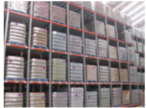
Pallet flow racking systems are a FIFO (First In First Out) dynamic storage system. Gravity flow racking maximizes storage space by minimizing aisles.
